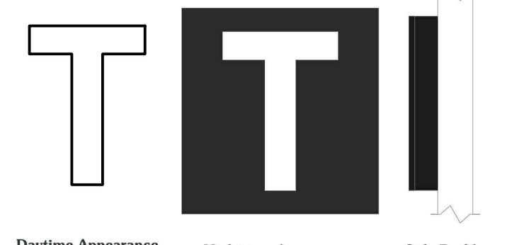
For Dark Colored Building Backgrounds | Letters to appear white during the day and illuminate white at night.
