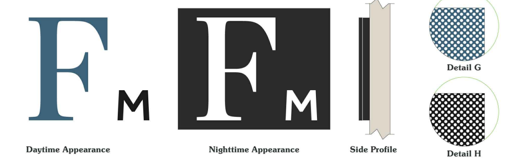
For Light Tone Building Backgrounds | Letters to appear blue and black during the day and illuminate white at night.
